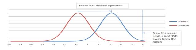
As shown above, when a parameter drifts from centre, the probability of an OOS increases.
